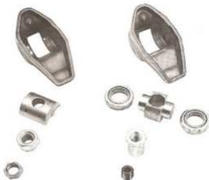
Stock Rocker Arm Assembly On Left. Ford Competition Rocker Arm Assembly (DOZX 6A585-A) On Right.
